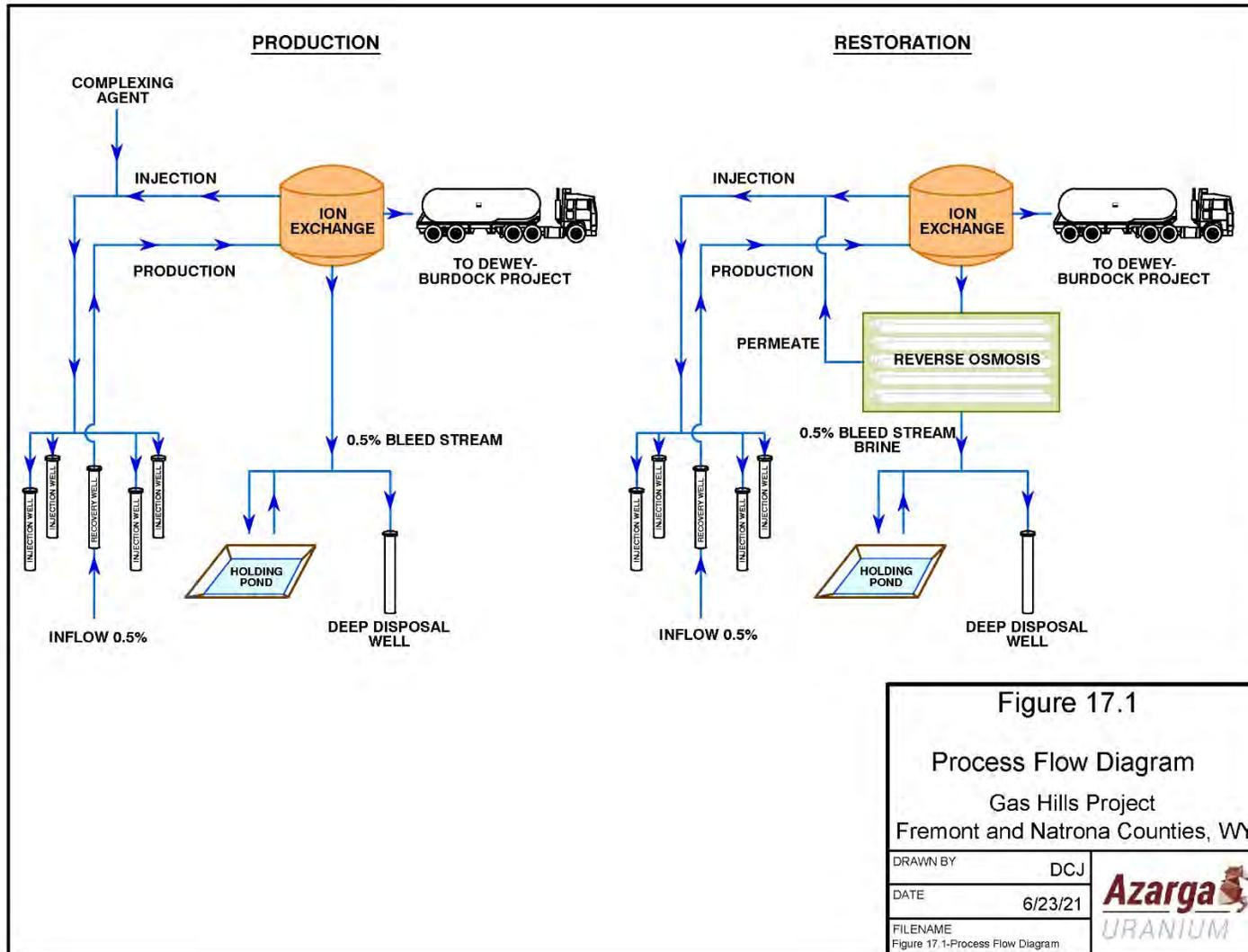
re injection. A low-volume bleed is permanently removed from the lixiviant flow to maintain an inward gradient within the wellfields. The wellfield bleed is disposed of by injection into an Underground Injection Control (UIC) Class I Deep Disposal Well (DDW). See Section 17.4 for a detailed description of the planned wastewater management system.
